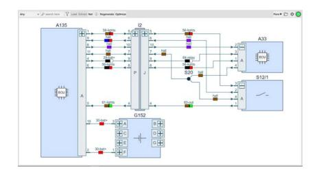
Unlike development ECAD systems and paper maintenance manuals, incremental schematics reduce the clutter of unnecessary detail, while highlighting key data to significantly accelerate development and debug. The views can be modified and transformed as the engineer moves around the system, with important information actually displayed on the schematic, for example, power distribution, component detail, and other nomenclature.
